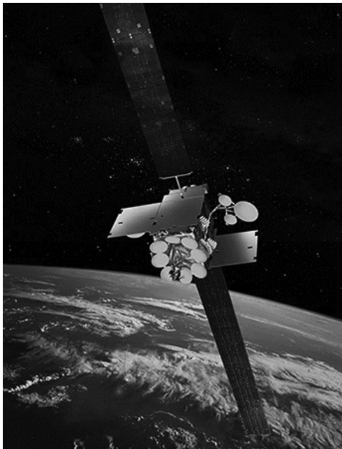
Figure 2. Inmarsat-5, a Boeing 702HP high throughput satellite
