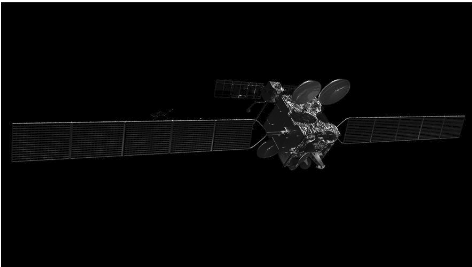
Figure 1: Depiction of a Servicer spacecraft (rear) docked to a telecommunications Client (front) and providing life extension services.
